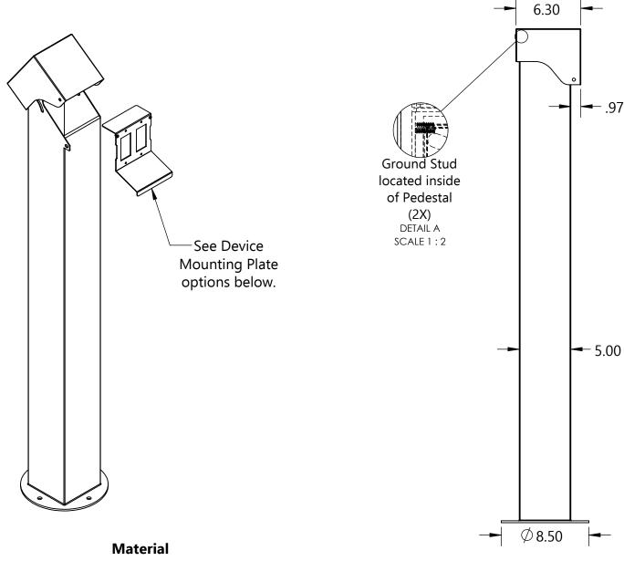
14 Ga. 304 Stainless Steel: Pedestal Body, Cover, Device Mounting Plate 7 Ga. 304 Stainless Steel: Integral Base
