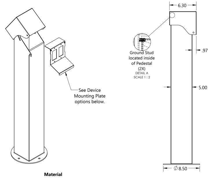
14 Ga. 304 Stainless Steel: Pedestal Body, Cover, Device Mounting Plate 7 Ga. 304 Stainless Steel: Integral Base
